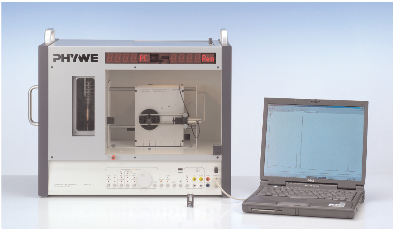
Fig. 1: Experimental set-up for the analysis of X-rays
