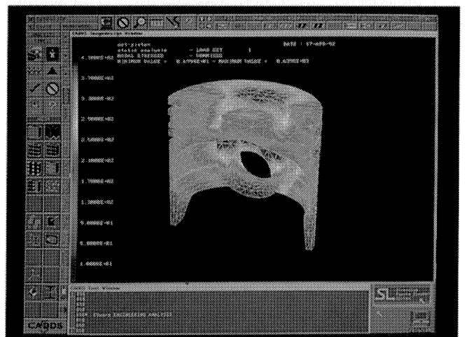
FIGURE 1 8 3D Design Model Used for Engineering Analysis
